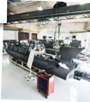
JFD Sweden's hybrid surface and subsurface vehicle, Seal Carrier , for military special forces.
