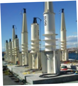
Wave energy converter with linear generator from Sea-based .
