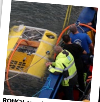
ROHCV , remotely-operated underwater vehicle from Saab for environmentally-friendly cleaning of ships' hulls without the need to drydock vessels.
